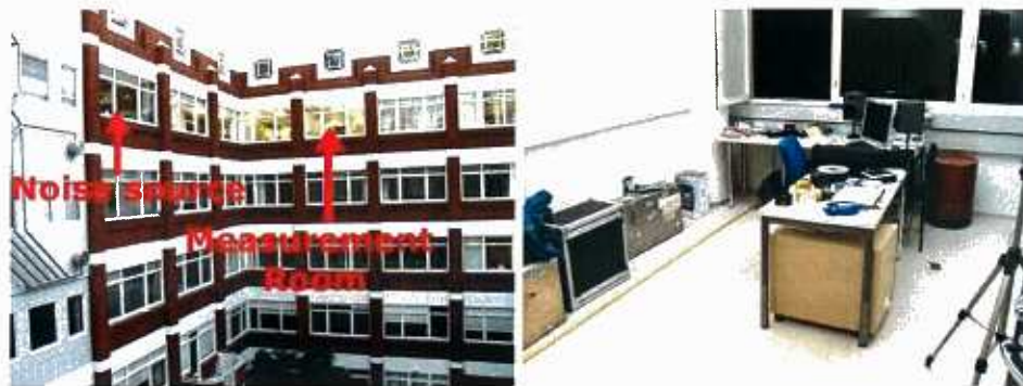
Figure 4 Left) Inner yard in Case 1. The locations of the source and measurement rooms are indicated. Right) Photo of the office room. The opened windows are shown behind.
