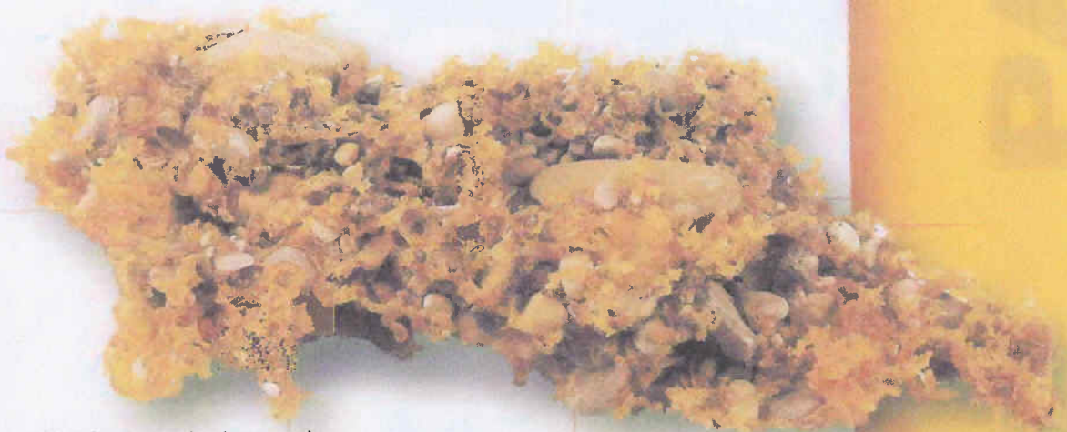
PA-Injektion in Lockergestein
